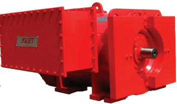
The Joliet Horizontal AC Drilling Motor delivers a continuous 1800 HP rating for mud pump and rotary table applications and boasts an impressive intermittent rating of 2700 HP for drawworks duty. The continuous rating is at 600 VAC, 1571 Amperes, 45.6 Hertz, 900/1800 RPM.
